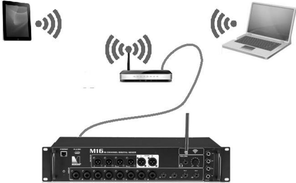
2) Mixed WiFi/Ethernet Remote Controllers using M28 Ethernet Port and WiFi Module
