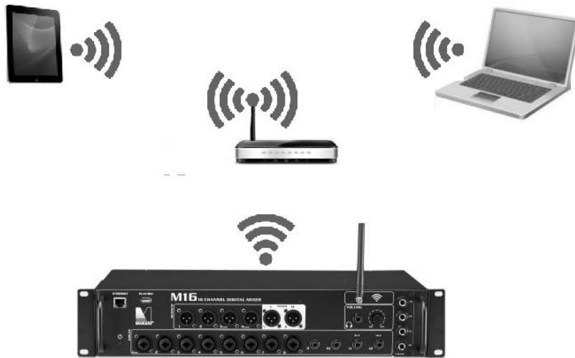
In WiFi Client mode the module connects to a WiFi network and supports DHCP client or static IP addressing. This way, both the M28 mixer and the remote control devices should be connected to an external WiFi router as shown below.
