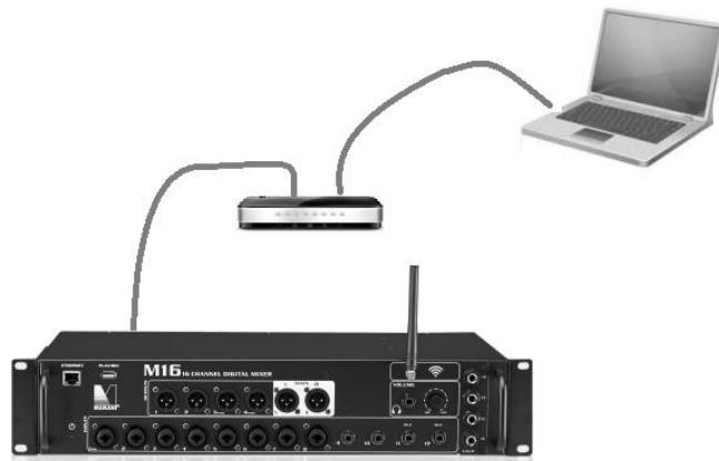
In this mode both Static and Dynamic IP addressing can be used since the M28 ethernet controller has DHCP client capability. Up to 10 remote controllers can connect the M28 at the same time.
